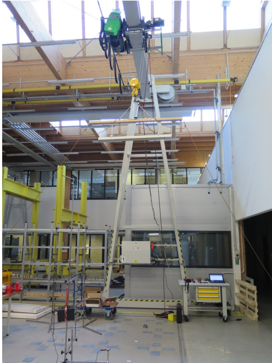
Figure 4-1 Radiant panel Ecosun hung on the crane in the measuring area
