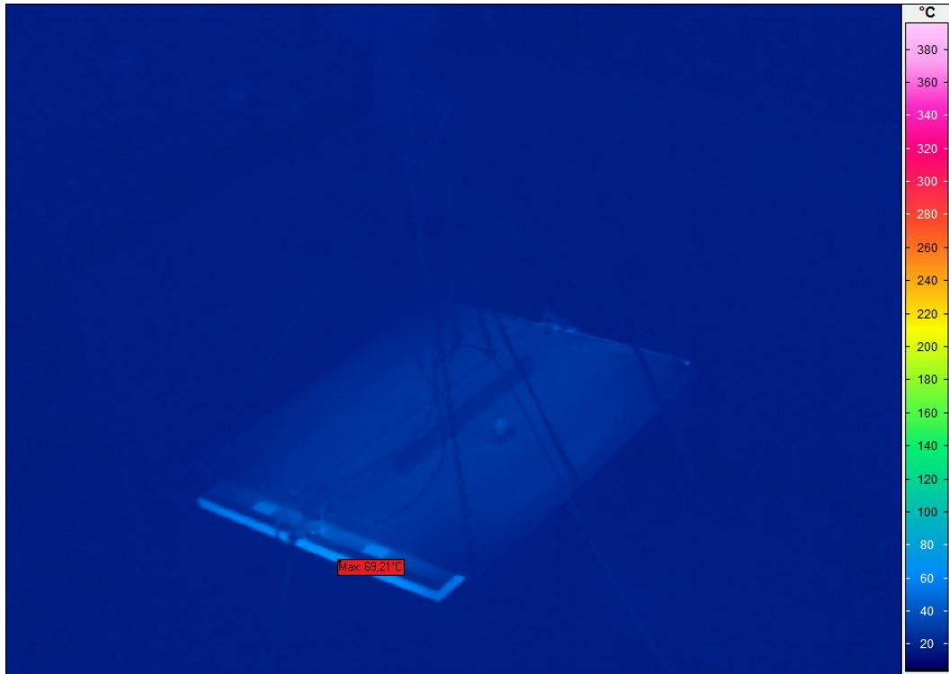
Figure 3-24 Thermal images of front area and rear cover of panel Ecosun 1000 U
