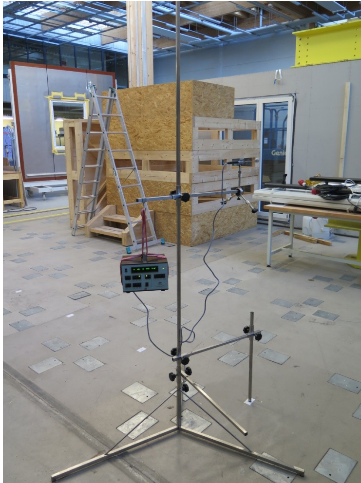
Figure 4-4 Tripod with radiant asymmetry sensor and Indoor Climate Analyser located in one point of measuring mesh (white marks on the floor)
